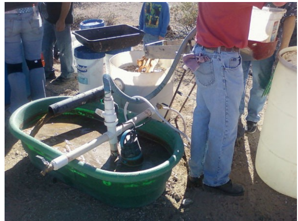
Re-Circulating Pump For The Sluice
